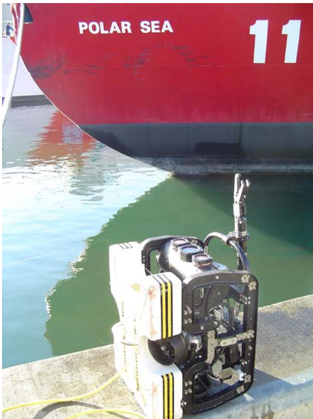
Figure 9. OCROV with Sample Collection Tube, HID Lighting and Mechanically Scanning Sonar
