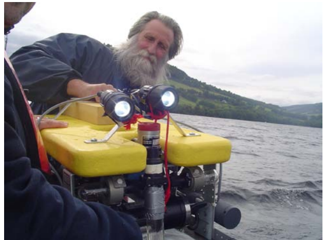
Figure 9. OCROV with Sample Collection Tube, HID Lighting and Mechanically Scanning Sonar
