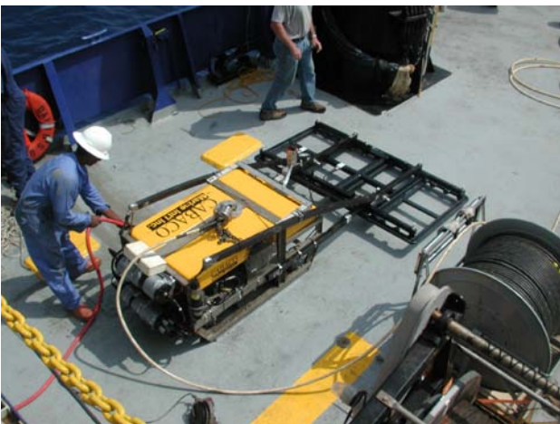
Figure 5a. OCROV with Pipe Tracker
