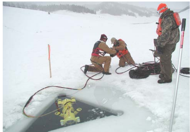
Figure 14. SeaLion Inspecting Ice-covered Reservoir
