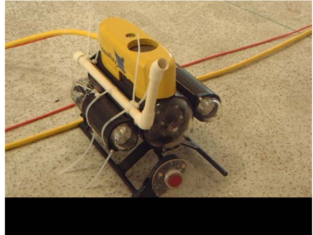
Figure 6. Micro-OCROV with Ultra-sonic Metal Thickness Gauge Attached
