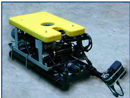
This Outland 1000 was deployed into a 400 foot deep and 8 foot diameter fresh water surge shaft in order to perform four different tasks: Turning 14 lb bolts, cutting hoses, cutting wires, and observing cement operations. While on site, it also removed 17 lbs of debris.
