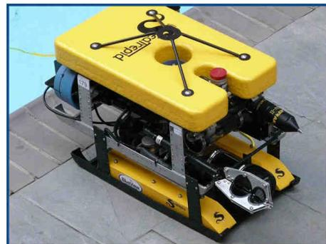
A custom Outland 1000 with an Imagenex 852 mechanically scanning sonar, BlueView multibeam sonar, cathodic potential probe, and modified Seabotix grabber. This system was customized for an inspection job in very low visibility.
