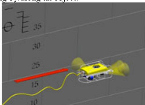
ROV swimming a hull with side-facing camera (Graphic by Benthos, Inc.)
