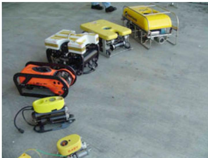
Size Comparison Between ROV Systems Tested
