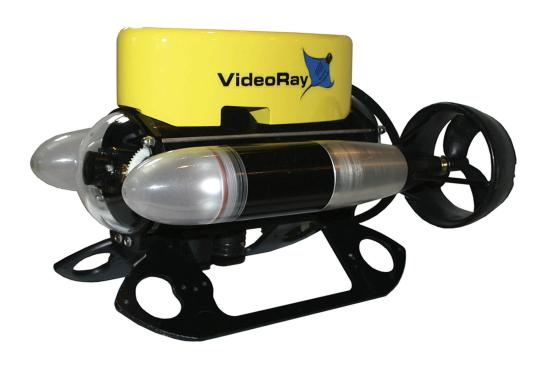
The SeaTrepid VideoRay PRO 3 GTO is an observation class ROV system capable of obtaining information when size really does matter. This system can fly through flooded pipelines, portholes, doorways, or other openings of 12 inches and greater to gather information quickly and efficiently. Due to the system size, it can easily be loaded aboard a helicopter to provide immediate response capabilities for nearly any application.
