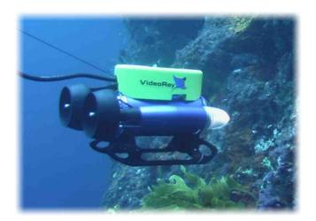
Due to the small stature of the VideoRay ROV, it is perfectly designed to inspect inside shipwrecks and other subsea structures. SeaTrepid personnel have used this system to inspect the USS Arizona, municipal water tanks, and as a reconnaissance tool for divers within fallen structures to help ensure their safety.
