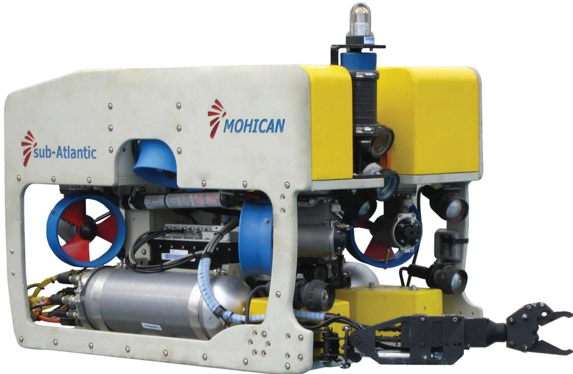
**The SeaTrepid Mohican Mid Class ROV offers a truly versatile, professional ROV system suitable for offshore use. Its size provides a stable platform for high quality video and sonar surveys, and its enhanced propulsion system allows it to continue working in high current conditions that could stop other ROVs.**
