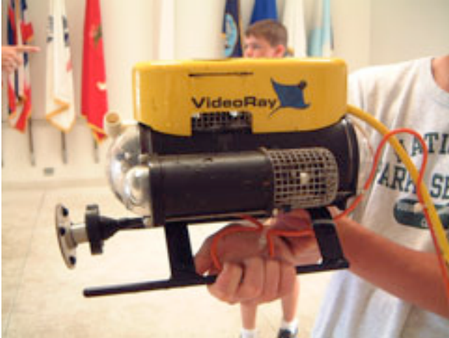
VideoRay with universal joint for mounting of Cygnus IV gauge (Photo by Bob Christ)
