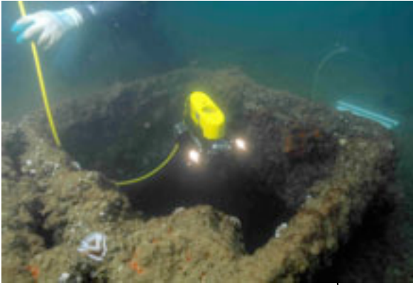
VideoRay entering hatch penetrating into 3 rd deck for oil analysis and metal corrosion analysis (Photo by Brett Seymour, NPS)
